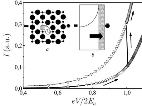
Figure 2: Expected current-voltage characteristic of tunnel junction as a result of transition (at  $V = V_c$ ) of barrier surface layer into metallic-like phase; triangles correspond to the “equilibrium” characteristics; the insets show schematically an oxygen ion jumping to a vacancy (a) and a partial metallization of the tunnel barrier due to diffusion of oxygen ions
